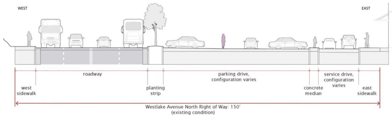
Figure 2. Westlake Avenue North Existing Example Cross Section.
